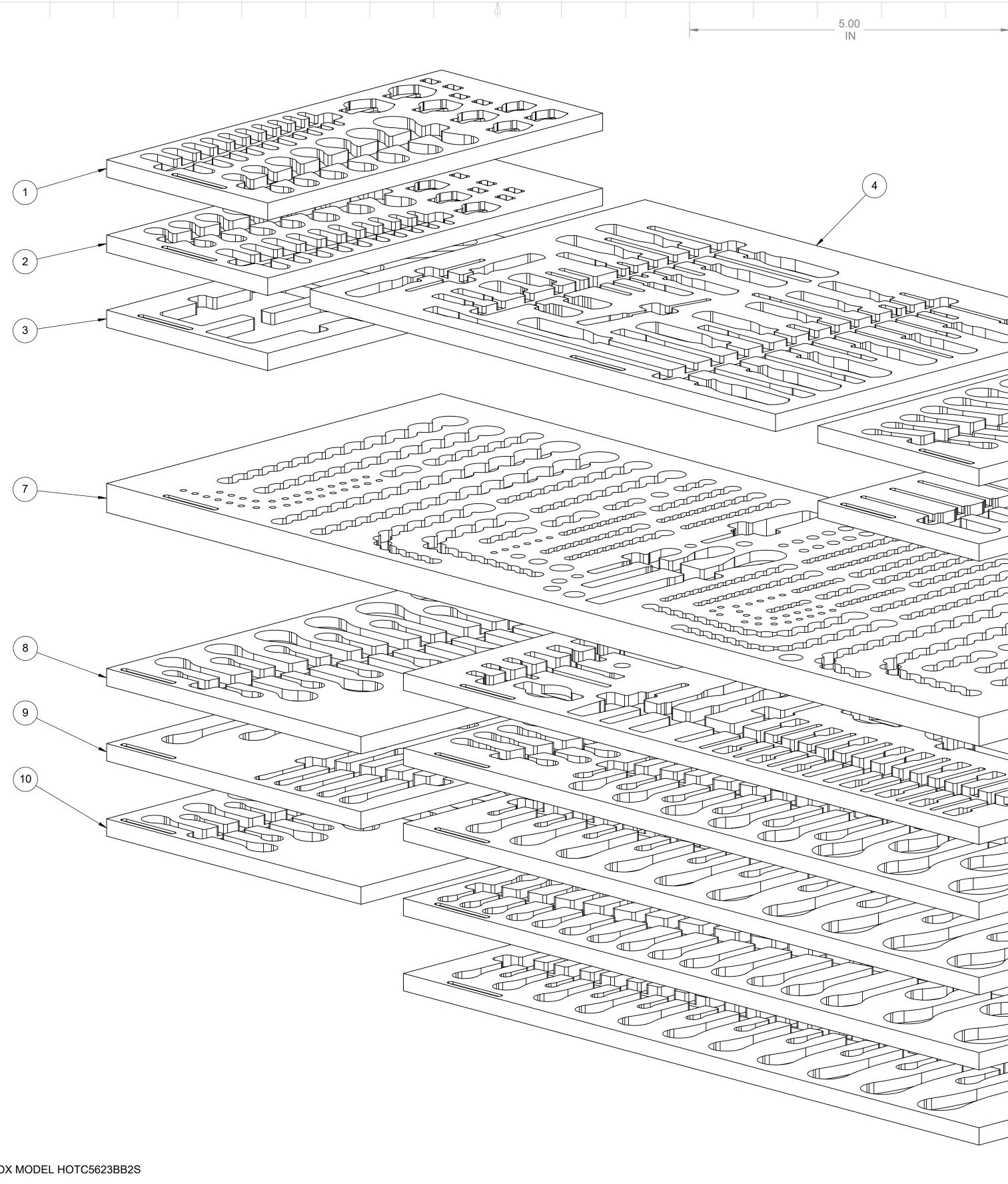
NOTES: 1. ORGANIZERS FIT THE HUSKY 922-PC SET H922MTSPO 2. DRAWER SIZES BASED ON MEASUREMENTS FROM 56-INCH, 23-DRAWER TOOLBOX MODEL HOTC5623BB2S
